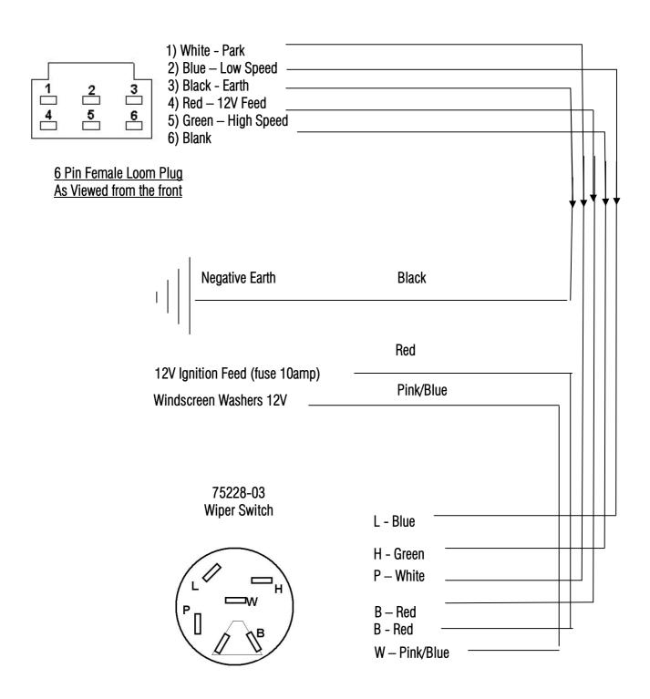
Wiper switch system is 12V Positive Feed
