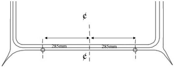
Locate And mark the centre of cowl windscreen opening width, measure out 285mm each side of centre, in the middle of *lower* radius as shown.
