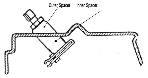
Wheelbox showing inner and outer spacer which will require some radius work to suit individual shaped cowls
